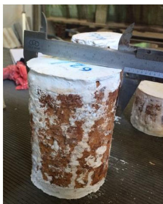
Figure 5, Applied capping on both side of MC sample
