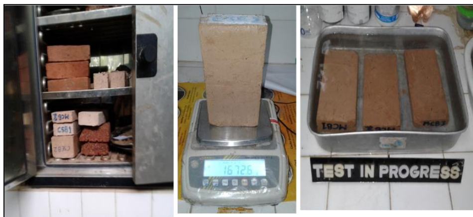
Figure 3, Water absorption test
