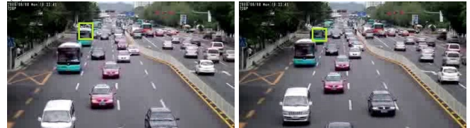
(c) After 20 frames (on left) using mean-shift the rectangle is moving away from the vehicle, while (on right) the mean-shift Kalman could track the vehicle.
