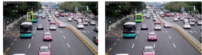
(d) After 60 frames (on left) using mean-shift the rectangle is away from the vehicle, while (on right) the mean-shift Kalman could still track the vehicle successfully.
