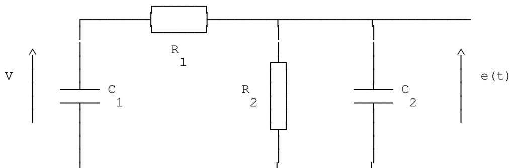
Figure 8.4 - Circuit to produce double exponential waveform
