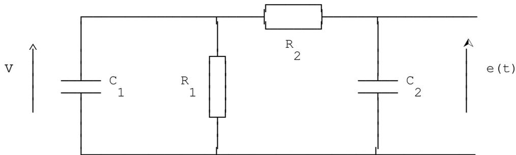
Figure 8.6 - Alternate Circuit to produce double exponential waveform
