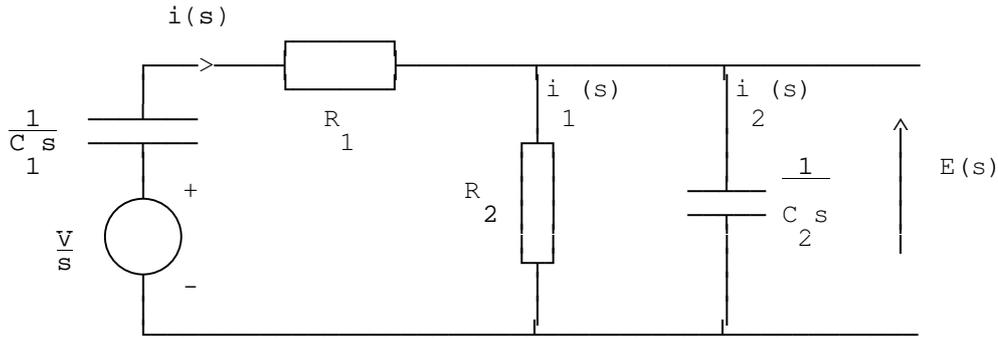
Figure 8.5 - Laplace equivalent circuit for double exponential
