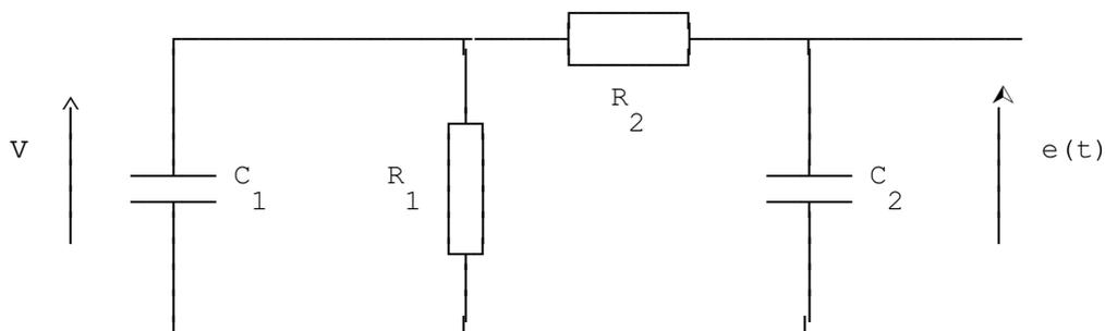
Figure 8.9 - Circuit to produce double exponential waveform
