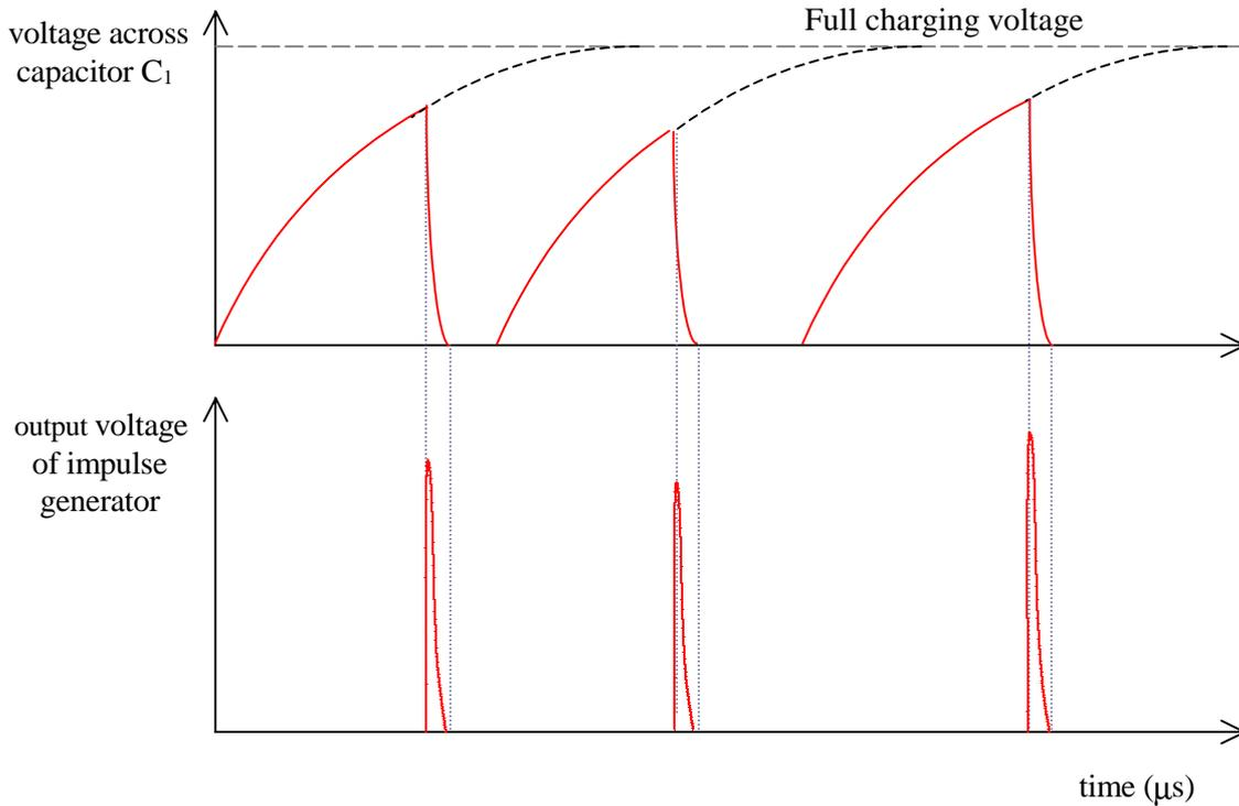
Figure 8.13 - Impulse generator waveforms for uncontrolled operation
