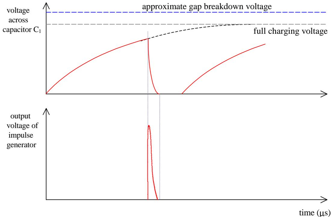
Figure 8.15 - Impulse generator waveforms for controlled operation
