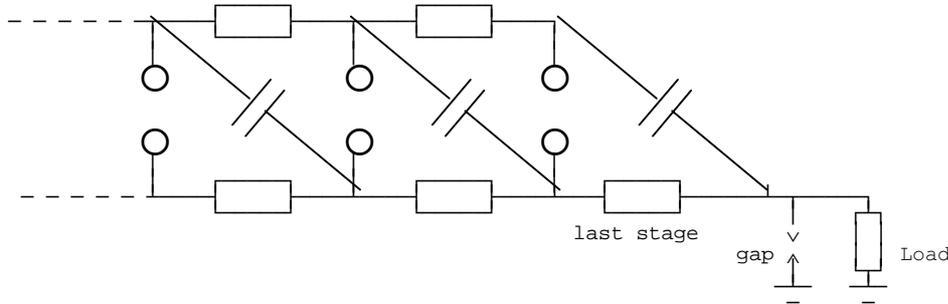
Figure 8.24 - Multi-stage impulse generator to obtain chopped waveform
