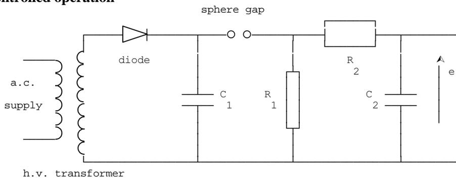
Figure 8.12 - Circuit for uncontrolled operation
