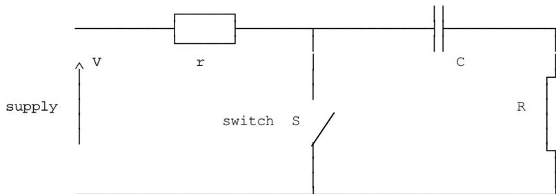
Figure 8.2 - Circuit to produce single exponential waveform
