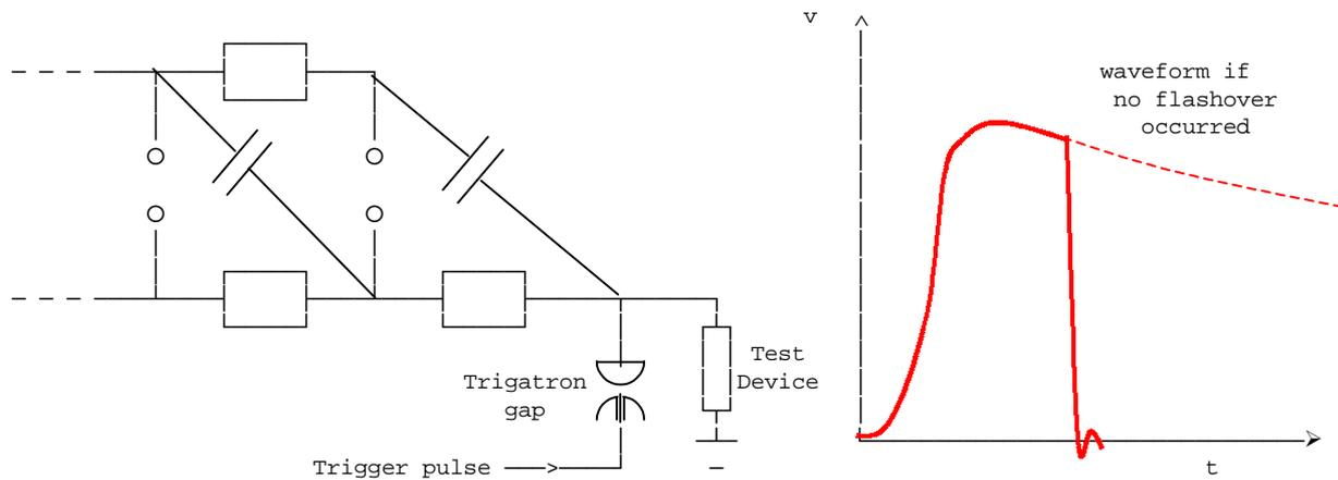
Figure 8.25 - Chopped waveform & Circuit to obtain chopped waveform
