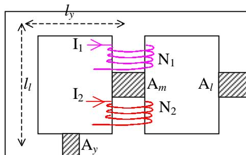
Cross section areas of the core, and the effective lengths of magnetic paths are indicated.
