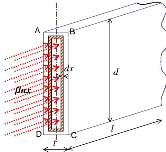
Consider the magnetic flux incident on the face ABCD of the cross-section of a lamination of thickness  $t$ . [The thickness of the lamination has been grossly exaggerated to show details of eddy current paths].
