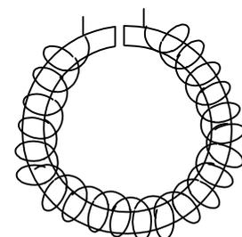
Let the cross section the core (and air gap) be  $A$ , the length of the magnetic path be  $l_m$  in the magnetic material and  $l_a$  in the air gap.
