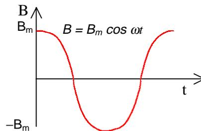
If the flux is alternating with flux density  $B = B_m \cos \omega t$ , then eddy currents will establish themselves round the periphery, as shown shaded on the diagram.
