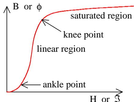
The terms, *ankle* point and *knee* point are used to define the curve as the diagram looks quite a bit like a bent leg with the ankle and the knee occurring in those positions.
