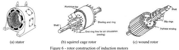
In the three phase induction motor the stator carries a 3-phase winding fed from a 3-phase supply. The stator windings, when supplied with 3-phase currents, produce a magnetic flux which is of constant magnitude but which revolves (or rotates) at a constant speed (at synchronous speed). On a 50 Hz supply, the synchronous speed for a 2-pole machine is 3000 rpm and for a 4-pole machine is 1500 rpm.
