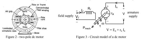
The dc motor needs slip rings or split rings (commutator) on the rotor shaft and a set of brushes positioned over them to supply the armature winding. [symbol for the armature basically shows the rotor and a pair of brushes]
