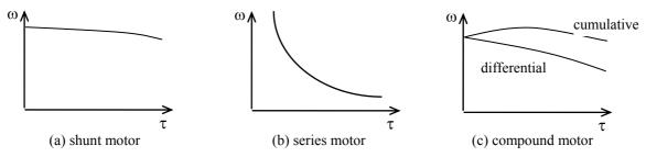
Figure 5 - Speed-torque characteristics of dc motors
